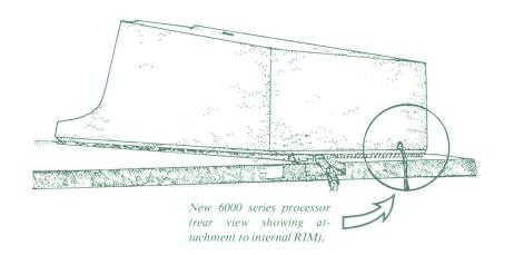
The new internal RIM offers several advantages. The bulky external RIM is eliminated, saving space and speeding installation. The total length of the I/O bus cable is reduced, and an additional power outlet is left free for other uses.
